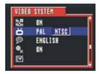
3. Then press the LEFT/RIGHT button ( ) to select NTSC/PAL. Press the SET button to confirm your selection.
